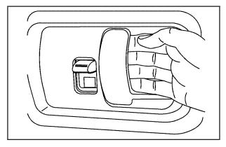
To open the front portion of a 60/40 door from the inside, pull the handle toward you and push open the door.
